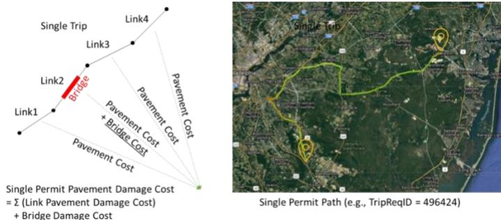
Figure 1: Pavement damage cost calculation procedure of a single overweight permit trip.
